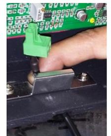
3. Place the wire for the power supply up through the middle hole of the base of the tower. Attach the plug into the connector marked "P" for power on the electronics board. Again be sure your transmitter power supply is plugged into the transmitter tower and the receiver power supply into the receiver tower.
